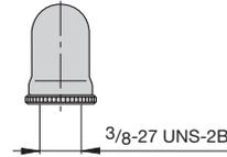
**Front panel water splash cover, transparent with special knurled nut**
